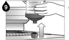
When the selected dispensing period of the Pulsarlube E has completed, remove the lubricator from the application.
