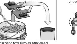
screwdriver, detach the PCB from the unit.
