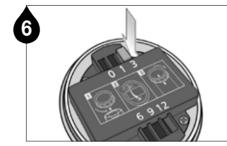
Firmly push the Mode Selector into the slot of the desired period.
