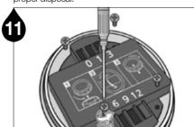
Unscrew the screws to remove the battery cover.
