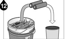
Remove the batteries.
