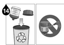
Warning Do not cut, puncture, or reuse lubricator.
